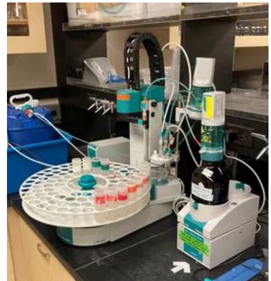
Robotitrator that is used to measure alkalinity of the water. Photo by: Hannah Hensel.
